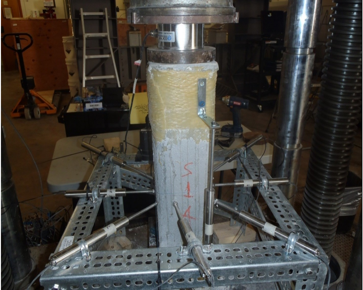
Fig. B-9: PBO-FRCM wrapped square column set up for testing
