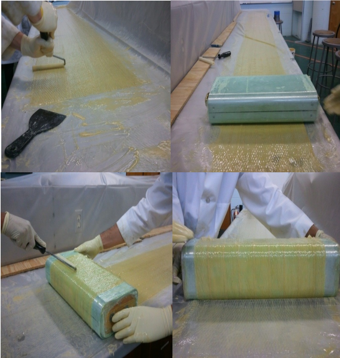
Fig. 2-3: Wet lay-up impregnation of glass fibers and wrapping of the aluminum
