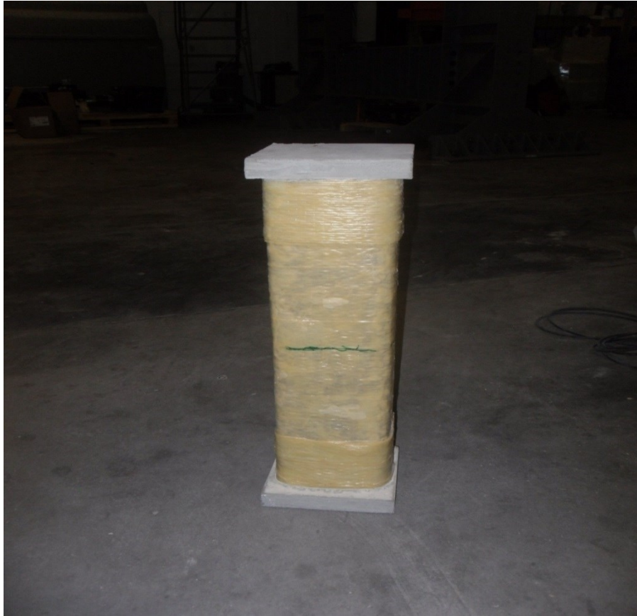
Fig. 3-2: Sample GFRP wrapped column
