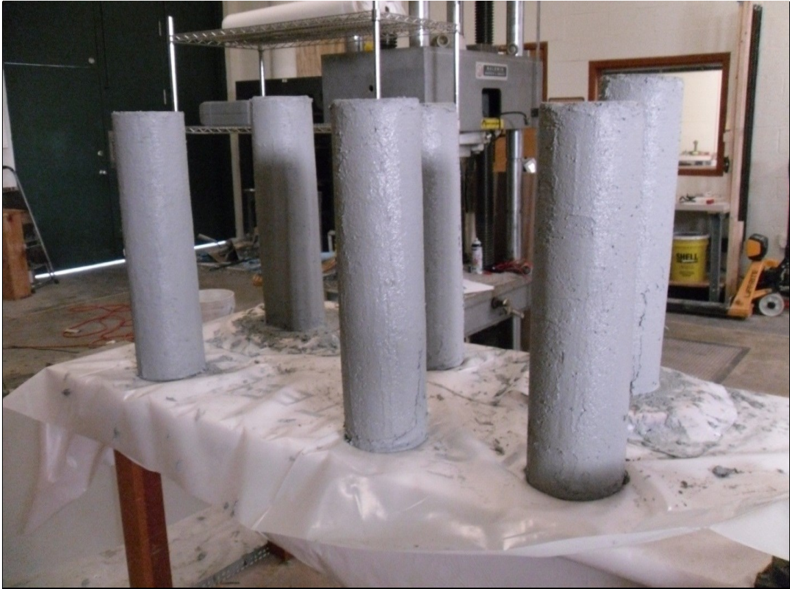
Fig. B-8: PBO-FRCM wrapped RC columns
