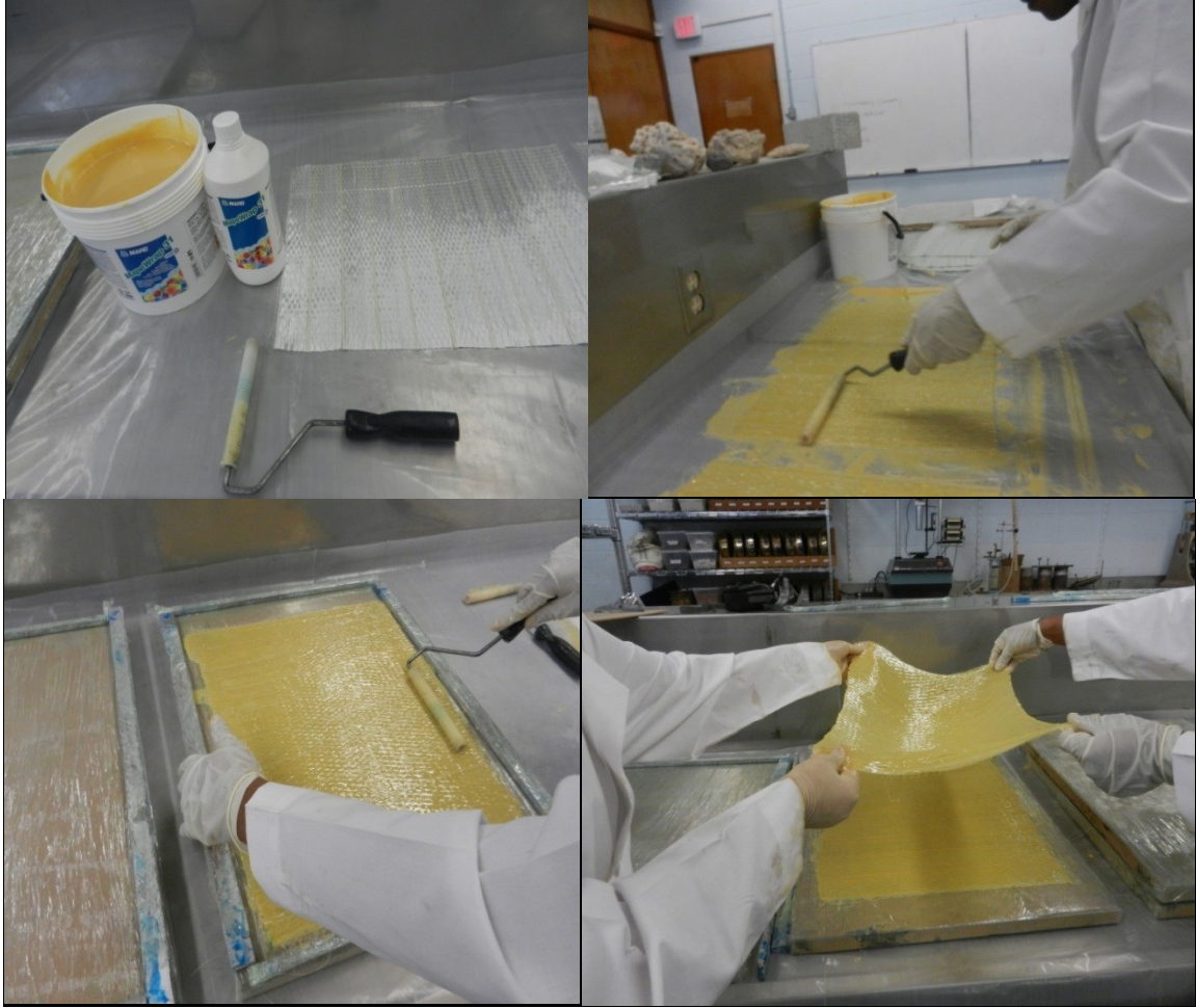
Fig. C-13: Preparation of GFRP flat coupons
