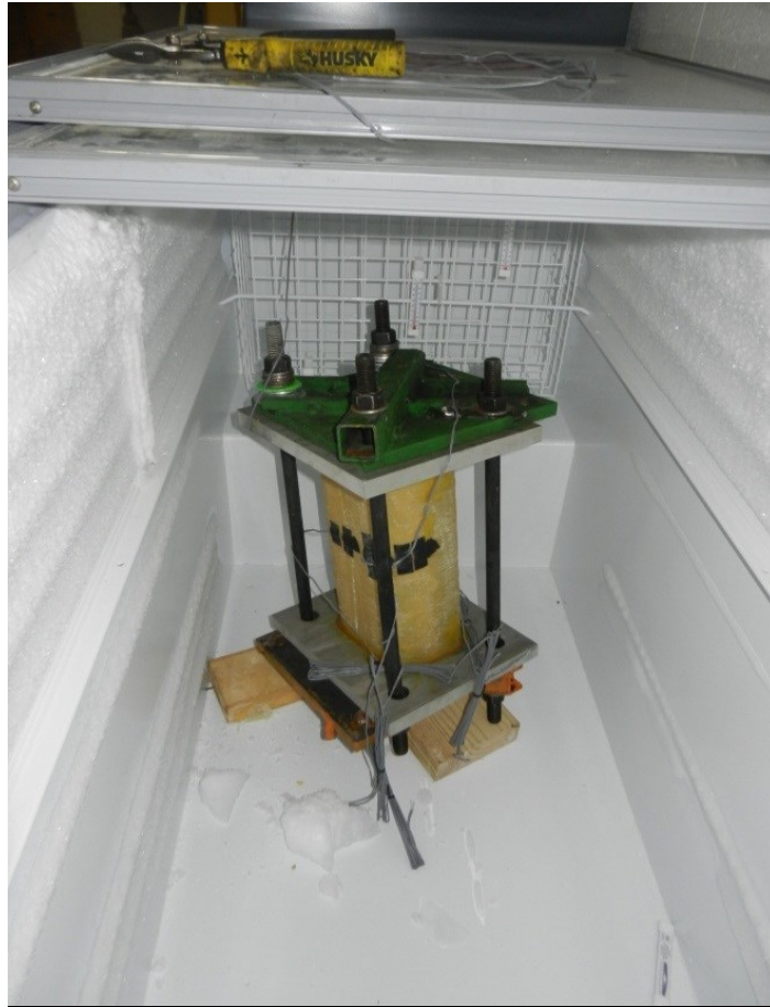
Fig. 2-4: Instrumented GFRP jacket inside the freezer
