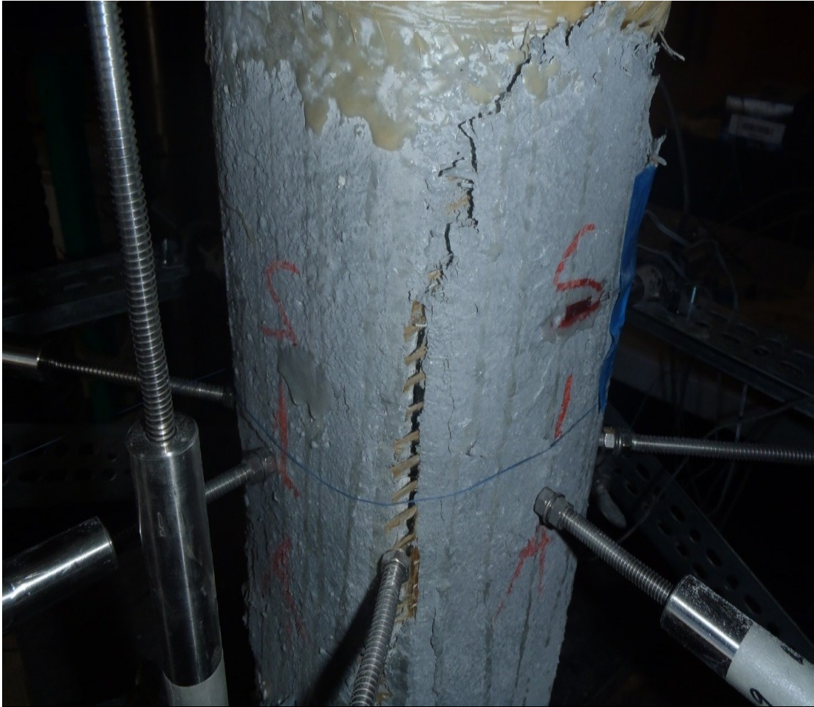
Fig. B-13: Failed PBO-FRCM wrapped square column
