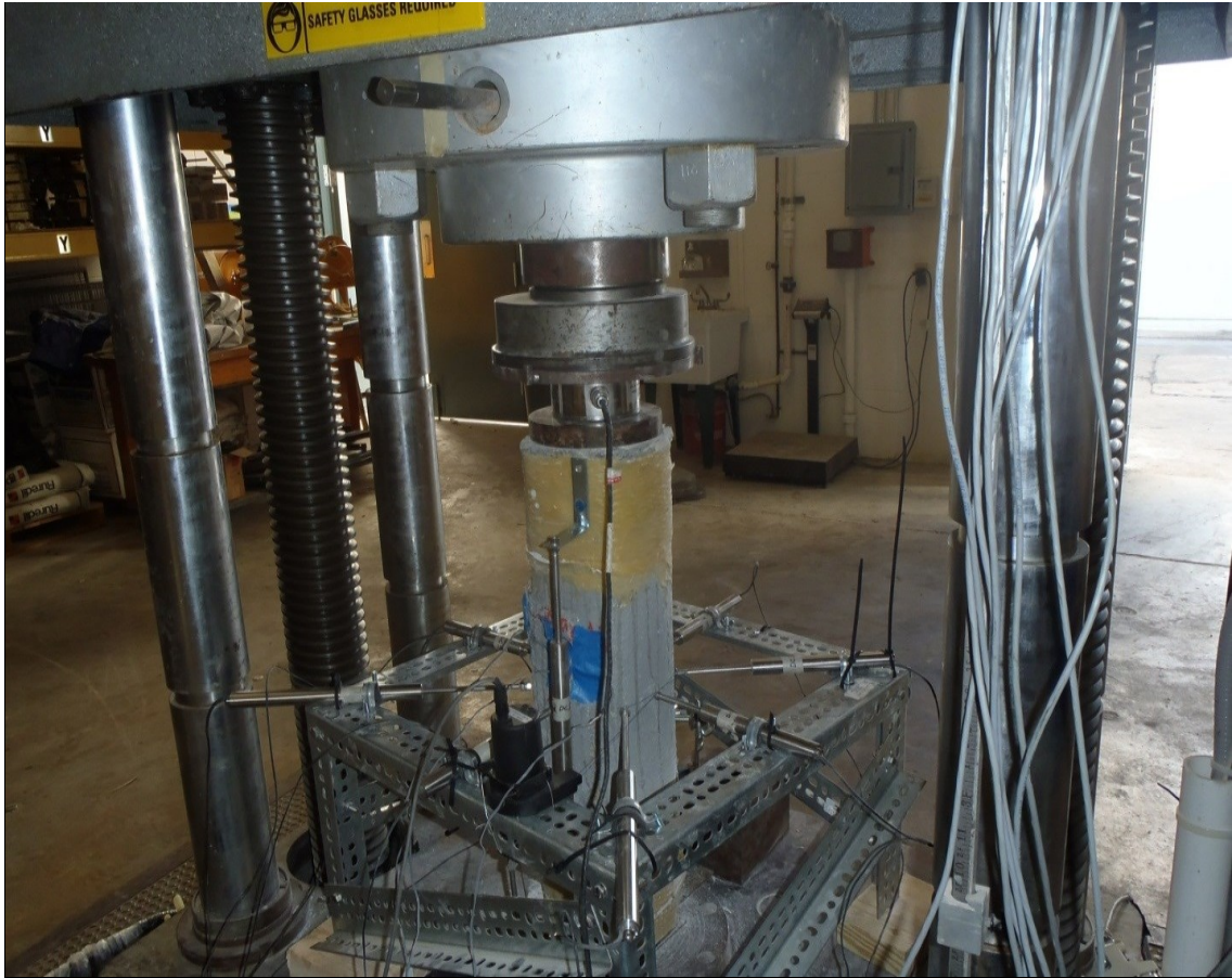
Fig. B-11: PBO-FRCM wrapped circular column set up for testing
