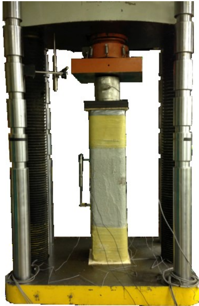
Fig. 4-3: Typical RC column specimen (square cross-section) before testing
